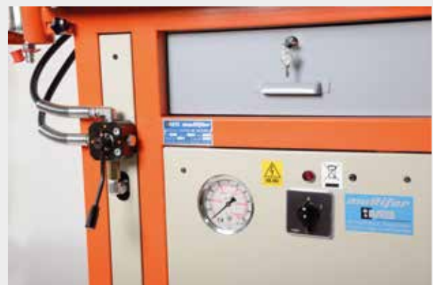
Branch valve with pressure gauge and general switch.
