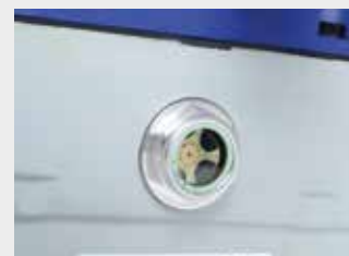
Porthole to check oil level
