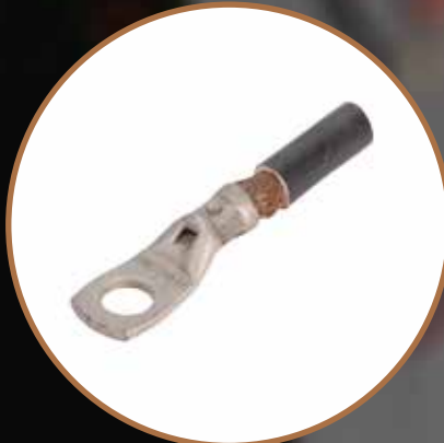
HEXAGONAL CRIMPING REALIZED WITH MANUAL TOOL
