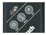
DSP 4-F with push button F for: phase sequence tests in ungrounded mains, frequency measurement or data hold
