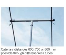
The MultiSafe TT OB is a two-pole telescope voltage tester for overheadlines of trolleybuses. Through his telescope design, the absence of voltage can be
