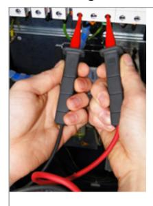
Different measuring lines for different voltages extend the application of the EXM. 72010 82010 Test lead for resistance Voltage test prods up to 1000 V AC / DC and current
