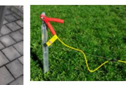
Ground connection, e.g. on the mast or with earth spike through clamp with strain relief
