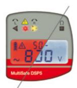
Colour change of the LCD lighting during voltage
